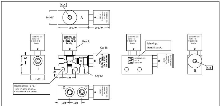
Key A: Illustrates Valve in housing cavity A, Doering Cavity C-8502 (8-2).
